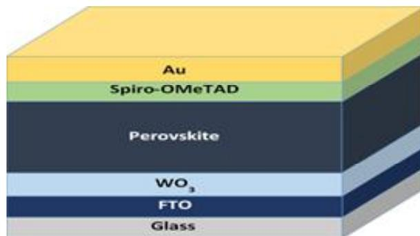
Fig. 2: Device Architecture of a planar PSC<sup>24</sup>
